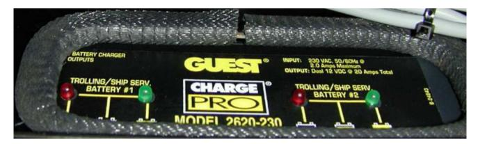
The above photograph shows the Guest 2620 charger as installed in the PowerTug It is located under the lid of the battery compartment. In-line 15A fuses are fitted. Only use replacements of the same type and rating.
