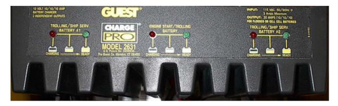
The above photograph shows the Guest 2631 as installed in the SUPER PUSHER. It is located under the hinged lid of the battery compartment. In-line 15A fuses are fitted. Only use replacements of the same type and rating.
