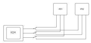
The 3 pole change over switch must have sufficient clearance and creepage allowance between IPD Relay channels in accordance with IEC installation requirements.
