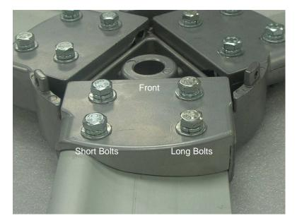
Use an industrial thread lock such as Loctite, or similar to prevent the bolts from working loose. Using a torque wrench, tighten all blade bolts to 14Nm.
