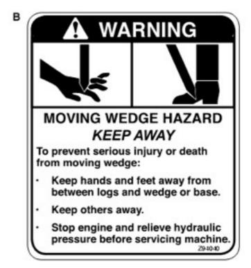
**REMEMBER** - If safety signs have been damaged, removed, become illegible or parts replaced without signs, new signs must be applied. New signs are available from your authorized dealer.
