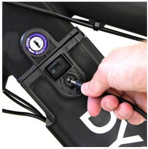
Charging can take place with the battery in the frame, or you can remove and charge separately.
