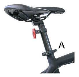
by loosening the hex screw located under the saddle. Adjust to the desired position then tighten.
