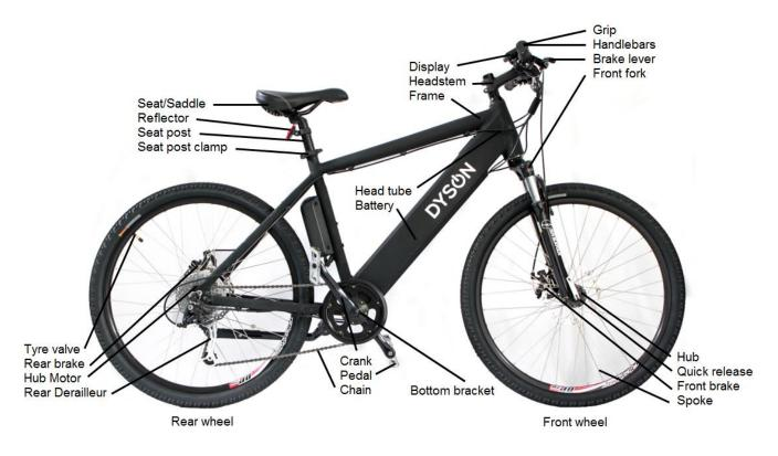
The e-bike serial number is engraved in the front of the head tube.
