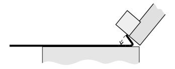
3. With thin workpieces, and/or where the lip is not too narrow, a more complete flattening can be achieved by following with magnetic clamping only:
