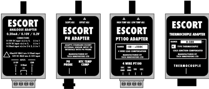
An Analogue Adapter is a device that plugs into any external sensor socket not dedicated to an external humidity sensor or pulse counting interface. An Analogue Adapter provides the functionality to let the logger connect to any type of sensor employing industry standard 0/4 to 20 mA or 0 to 10 Volt outputs. Specific adapters for PT100, Thermocouple and pH sensors are also available.
