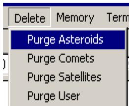
If you study the output in the Terminal window, you will see that ARGONAUT™ will send an “asteroid”, “comet”, “satellite” or “user” command, as appropriate, followed by “#Purge”, “#Write” and “#Quit” commands. ARGONAUT™ will display a “FINISH” message when the catalog purge is complete.
