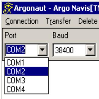
Ensure that the ARGONAUT™ Baud rate selection is the same as that on the ARGO NAVIS™. Then attempt to Connect to the PC COM port using the Connection pull down menu –
