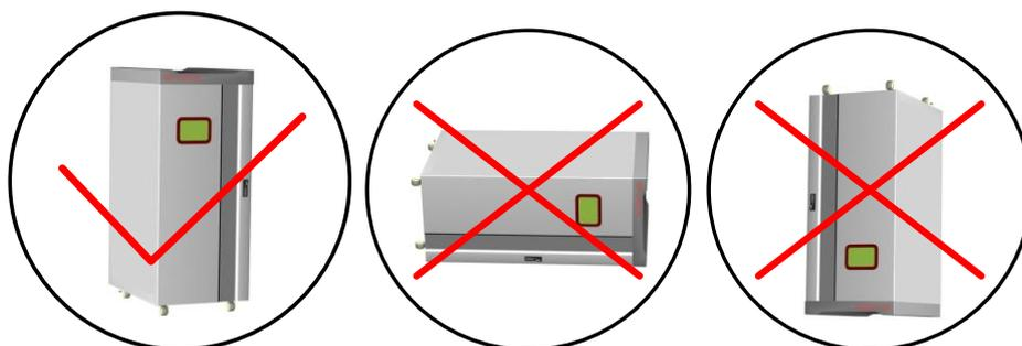
Fig 2.2 Correct placement of battery cabinet
