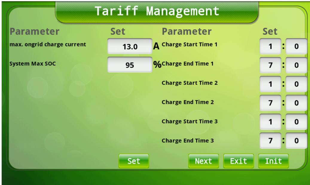
Fig 5.5 Setup interface 1 of tariff management mode
