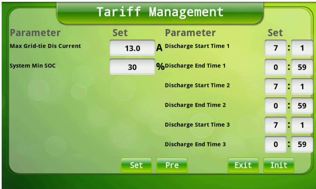
Fig 5.6 Setup interface 2 of tariff management mode
