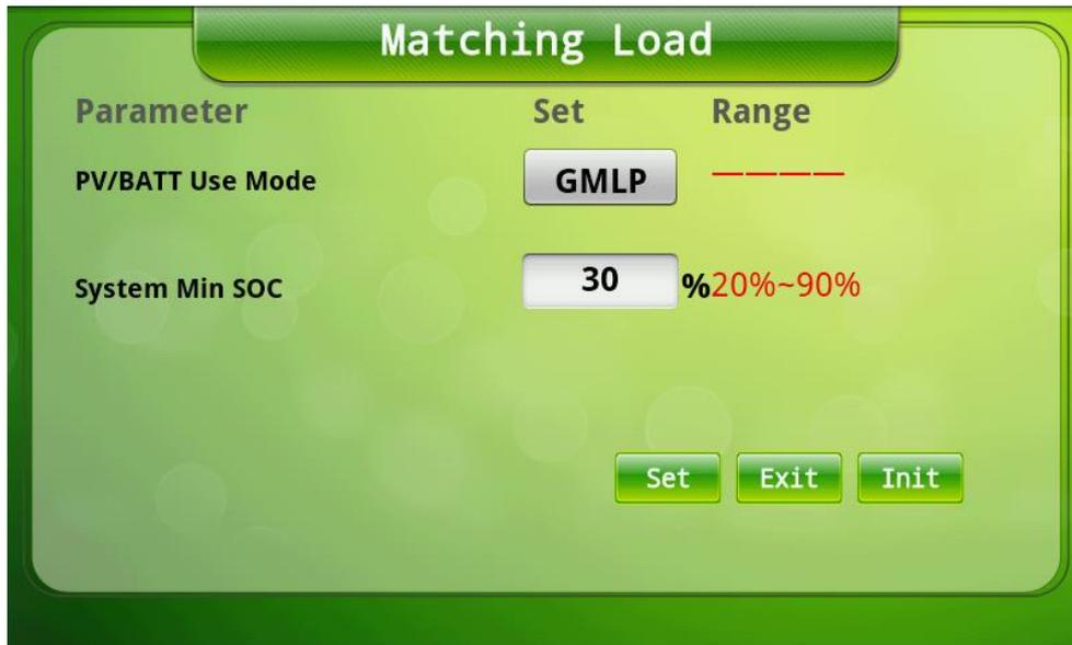
Fig 5.2 Setup interface of matching load mode
