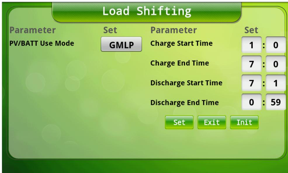
Fig 5.4 Setup interface of load shifting mode
