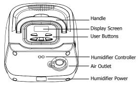
Handle: This handle is for lifting up the system.
