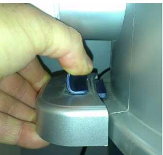
4 replace the dust bin & lock the latches
