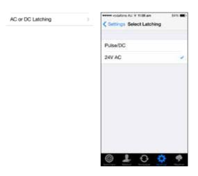
The WaterMe system has been designed to accept 24VAC/24VDC solenoids or DC latching solenoids. Most irrigation solenoid valves are 24VAC types. WaterMe has been uniquely designed for a modulating output circuit. It has been designed to drop the output voltage after turning
