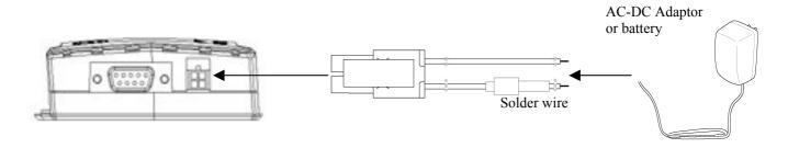
Connect the connector to the modem. The modem will turn on automatically.
