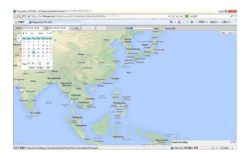
And then Click "Play", the system will load the history tracking and playback automatically, you can slide the blue "" button to slow to make the playback speed slower, and the right bottom window will display the event recoding (Stop time and period etc.), the server will keep the tracking data for 6-12 months.
