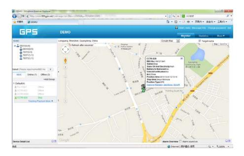
For the sub-fleet car, click the sub-fleet name, the sub-fleet car name will display in the left bottom window, also click the car name, the car location will display on map (For Example click sub-fleet TEST1, the car T1 will display, click T1, T1 location will display).
