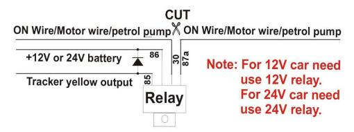
Attention: Turning off car engine is very dangerous when the car is moving, so we recommend install the relay to cut the start motor wire, this will make you can not remotely turn off the car engine, but you can make the car engine can not be started.
