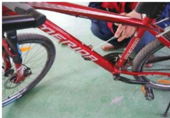
Remove screws for bottle holder from frame
