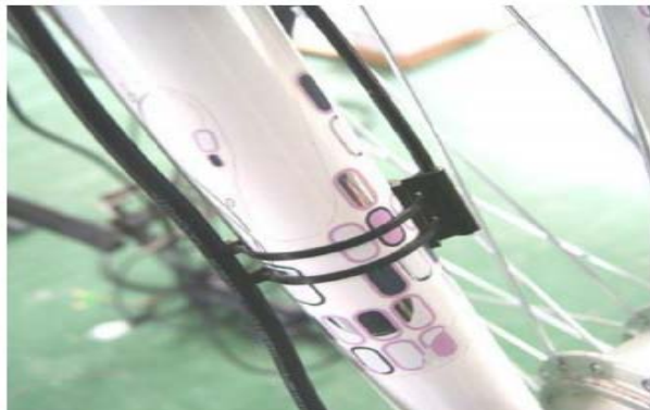
Mount the sensor to the fork using the rubber bands
