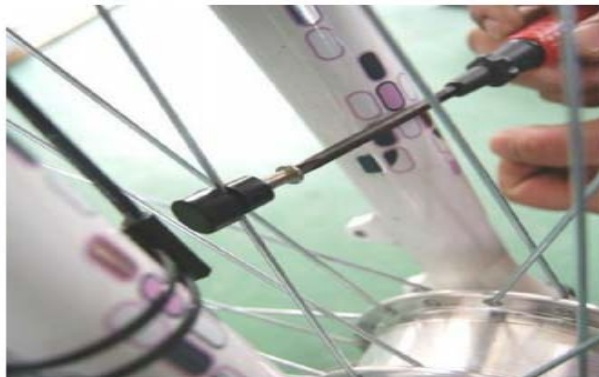
Mount the magnet to the spokes using a Philips screwdriver
