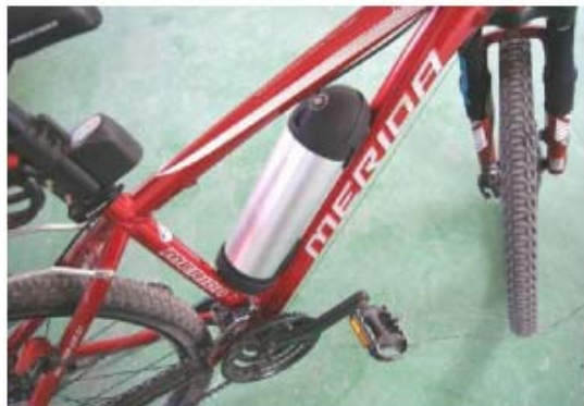
Put the battery into the case. And connect the battery to the controller
