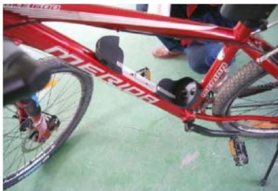
Use the screws to fix the battery holder to the frame
