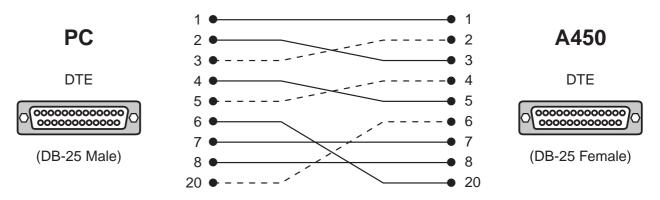
For reliable RS-232 line powered operation of the A450 use a cable with all pins connected as shown in the diagram above. However, the A450 internally ties CTS to RTS and DSR to DTR. This means that the diagram below is a minimum cable configuration for unpowered operation.
