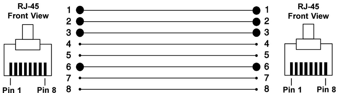
Figure 6-1 - A2200 ShareMate to A516 DataMate Cable
