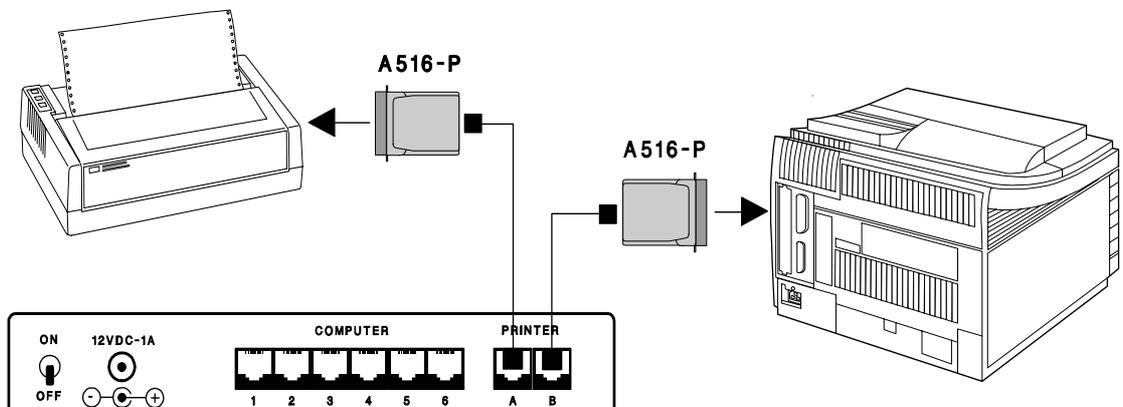
Diagram 3-2 - Connecting a Printer to the ShareMate
