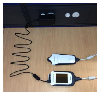
Fig 2.8 Display Power Supply Connection
