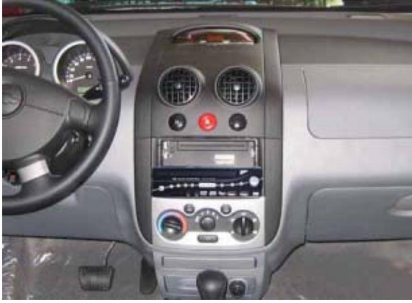
Above photo shows installed Car PC after unit has been installed into dash.
