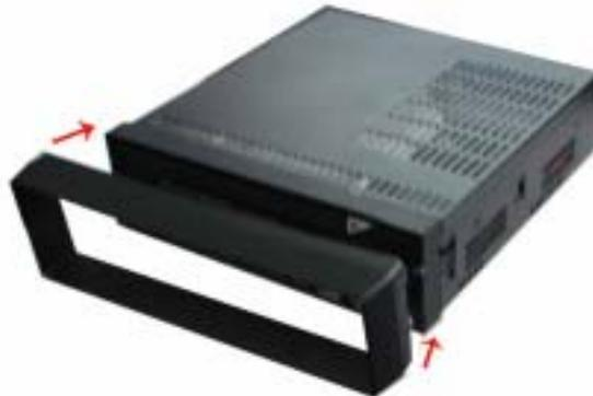
4.5 Slide the Car PC unit into mounting case after case has been installed
