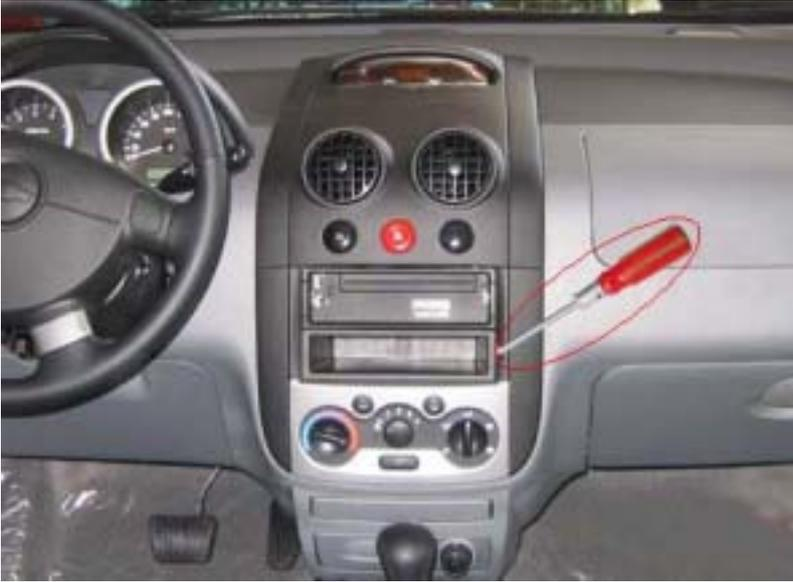
4.1.2 Gently push the mounting case into the mounting bracket.
