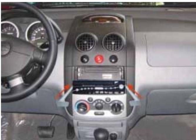
3. Remove key and begin removing the unit using “ side-to-side ” movements
