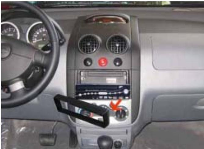
2. With an iron frame key, infix the key from the left and right sides of the mainframe
