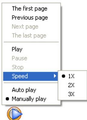
When the software is in “Board” mode, the icon with the blue play button (see pic to left) will be displayed at the lower left side of the screen. This button enables you to replay/pause the building of any page in any whiteboard file.
