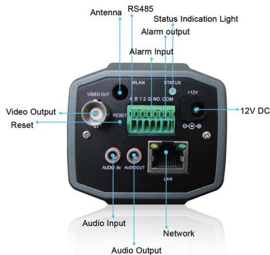
Picture 1 HD Box IP Camera Connection Diagram
