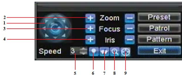
Figure 3. PTZ Control Interface
