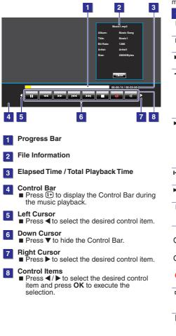
Use these control items on the Control Bar or these buttons on the remote control to control the music playback.
