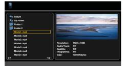
5 Press ▲ / ▼ to select the desired folder and press OK to open the folder; or press ▲ / ▼ to select the desired file and press ►II to start playback.
