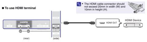
If the external equipment has DVI output, you can connect it to the HDMI terminal using a HDMI-DVI cable. In case of using the HDMI-DVI cable, connect analogue audio signal to RGB audio input terminal.
