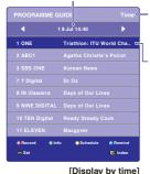
Press ▲/▼ to select the top bar and press ◀/► to change the display by channel.
