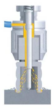
The use of cutting fluids is absolutely necessary when drilling with steel cutters. Always use the correct cutting oil intended for use. Other oils may provide insufficient lubrication under different temperatures.
