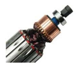
With regular use, the armature should be checked at least once per month. Look for visible damage or wear to the armature body and the commutator (commutator are brass plates which the brushes are touching).
