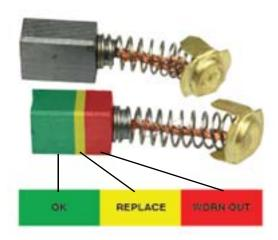
The motor on this machine has brushes. The brushes should be checked regularly to detect any abnormal wear.
