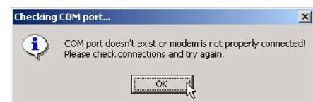
We suggest that you verify the connections between the TWIST GSM modem and the PC and between the modem and electrical wall socket. Ensure that the modem is switched on.
