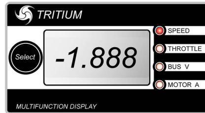
The motor controller uses PWM control when driving forward and current control in regen. This control behaviour can be observed using the Throttle and Motor Current values. If the user is driving forward, the Throttle display changes as the encoder is turned and Motor Current displays a fixed value. When changing into Regen, the Throttle value becomes fixed and the Motor Current reading will vary.
