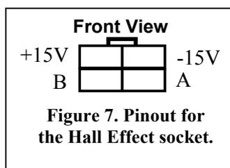
Figure 7. Pinout for the Hall Effect socket.
