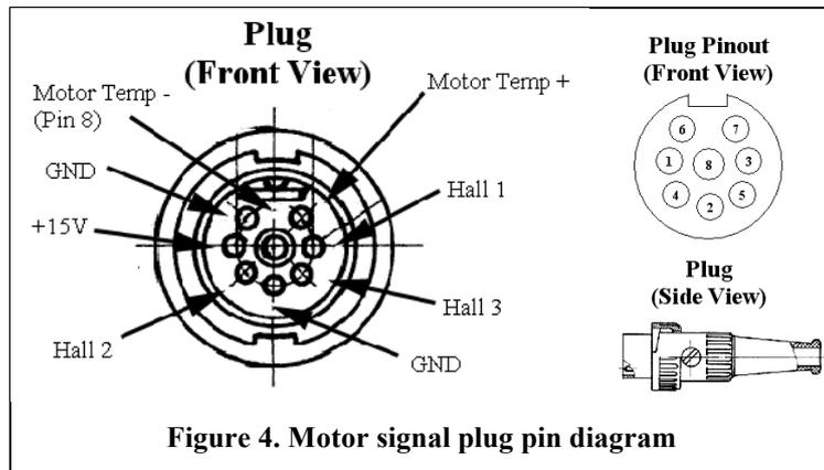
Figure 4. Motor signal plug pin diagram
