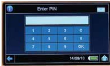
The IHD will ask for a pass code by displaying the key pad to enter the pass code; the factory default is 0000.
