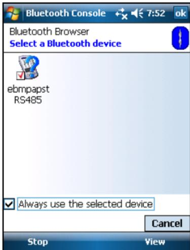
Here you have to enable *Always use the selected device* and tap on *ebmpapst RS485*. Close the message that appears afterwards. The scan will then run a little longer and shows this screen:
