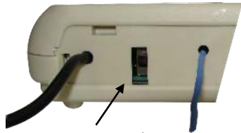
Power switch (Down is on)
