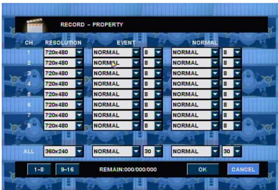
➤ resolution – set recording resolution for each channel.
