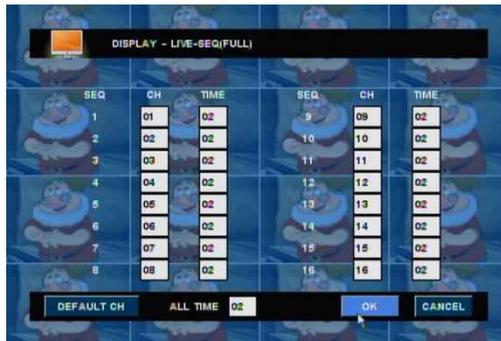
● **Screen display setup – live sequence scanning (quad screen)**
