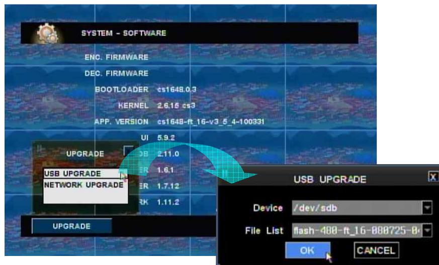
(6) Device – select USB device with firmware file.
