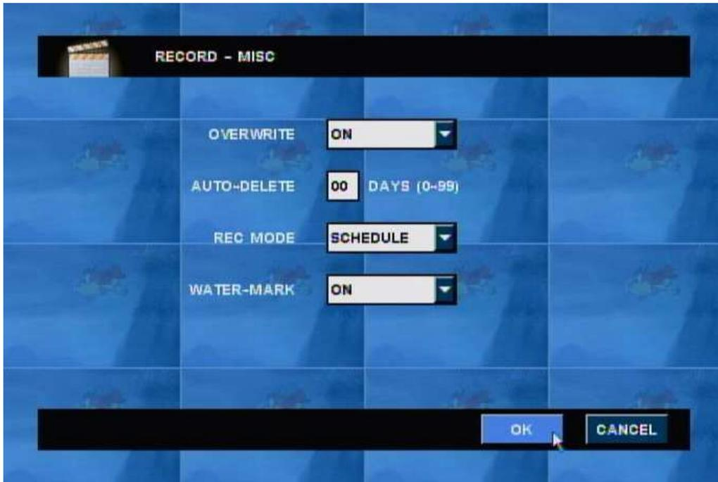
**Note)** when setting as ‘ON’ for ‘Water Mark’ option, all recording files are applied with watermarking, this recorded file can be checked at Backup Viewer if someone is altered or edited recorded file with intentional purpose.
