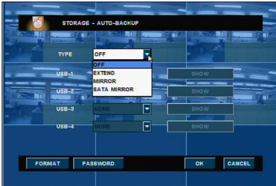
**EXTEND:** User can use EXTEND backup through connected USB external HDD.
