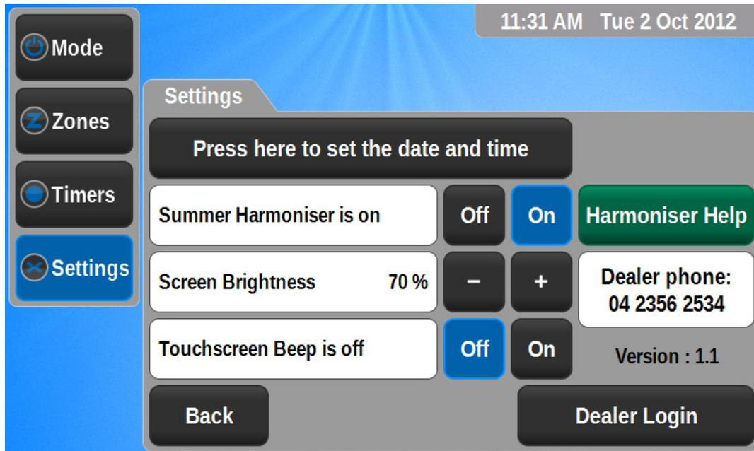
To adjust the system date and time press the button “Press here to set the date and time”
