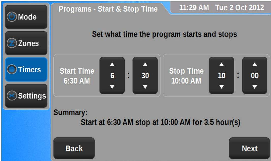
Enter the Start time for the program to start using the arrows on screen
