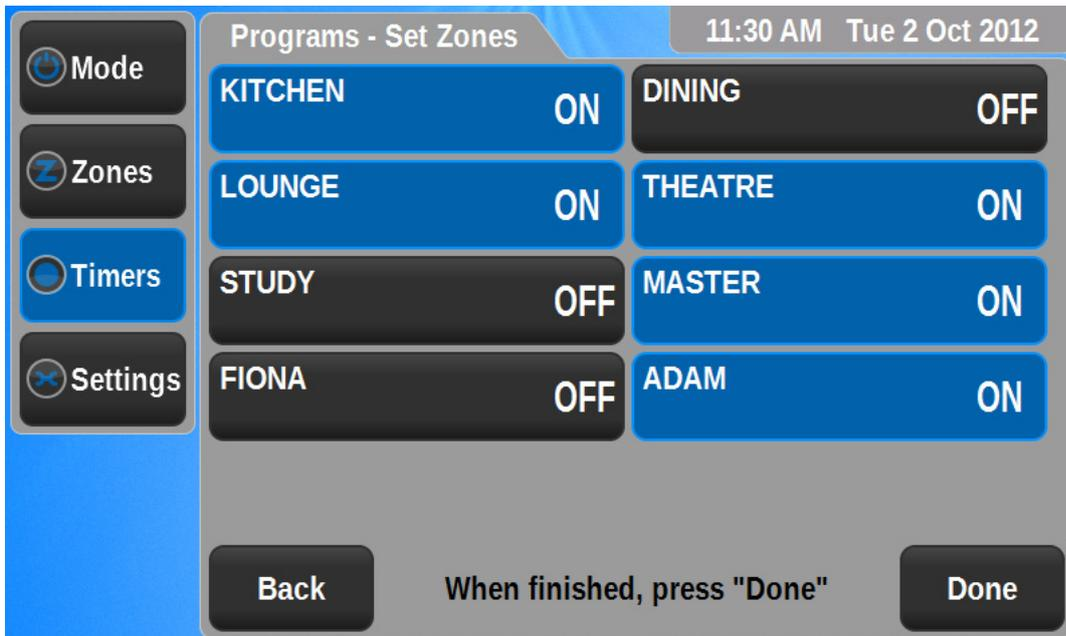
Press a zone to toggle between ON and OFF for the setting of that zone during the time the program is set to run
