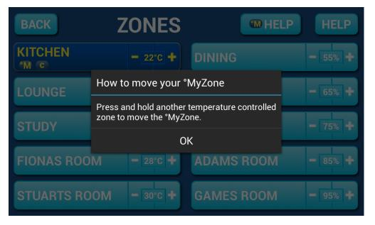
The MyZone can be identified easily, as the colour of the zone will change to DARK BLUE & display the **°M** symbol. In the example above you can see the KITCHEN is currently the active MyZone.
