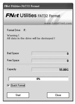
4. Click the *Quick Format* checkbox in the screen that appears, and then click the *Start* button. The utility formats the drive, and progress is shown in the progress bar. When complete, a pop-up appear to let you know formatting is finished.
