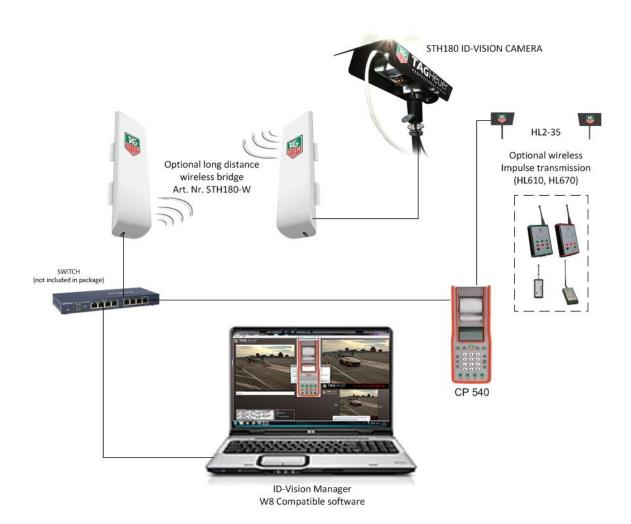
The wireless bridge option HL180-W allows a long range video stream transmission. With our Impulse radio transmission, it's the perfect combination in order to set the camera on place without visual contact.
