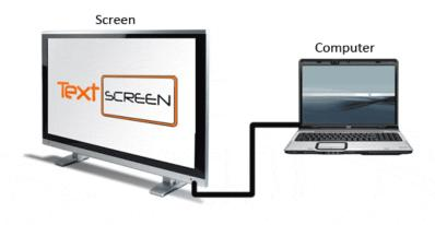
Once a cable is connected, ensure that the TV, projector or digital display is set to correct input channel relative to the cable input. E.g. If you plug your computer into the plug labelled 'AV3' ensure your channel is set to 'AV3'
