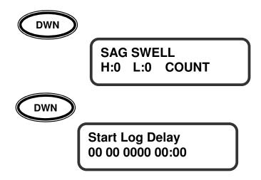
This Display if set at O or at any expired date and time will enable the logger to log as soon as it powered up. To set start delayed logging time see Setup Menu Start delay time. If the date and time is set to a future date time setting then logger will not log until that time has arrived.
