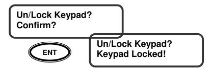
Once the keypad is locked the SPL will only display the MAIN Display and the SETTING Displays. The key lock takes effect when the setup program is exited.
