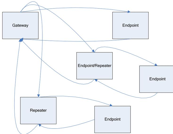
The next example depicts a standard Point-to-Multipoint network. From the Gateway, any data is broadcast to all three Endpoints, one of which receives it through a Multipoint Repeater. The data is in turn sent out of the serial port of each of the three Endpoint. The end device should be configured to interpret the serial message and act on it if necessary.
