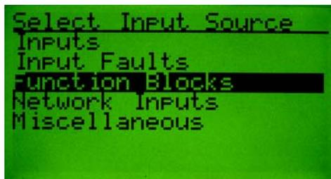
Use the **INC/DEC** keys to select the type of the source to assign to the Output. Press the **Enter** key when the desired type is selected. The following screen will appear (assumed "Function Blocks" selected):
