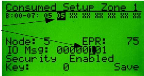
As mentioned earlier, use the **Sel** key to highlight the various ZIP configuration parameters for this zone. The following screen shows the "Security" field highlighted.
