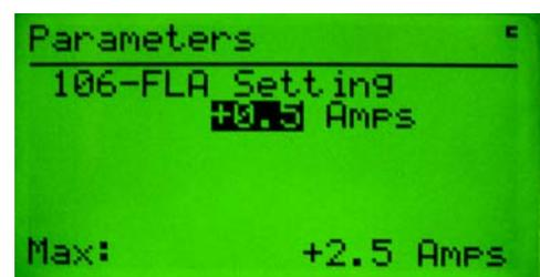
Pressing the **Enter** key will write the new value to the selected device. When a parameter value is selected, pressing the **ESC** key will deselect the parameter value and allow movement within the parameter list or group.
