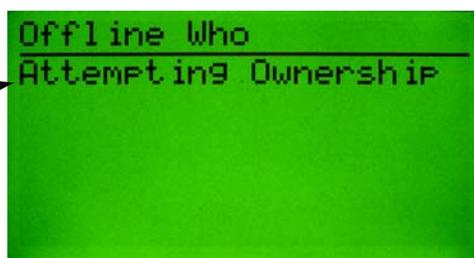
**Note:** It may take up to 10 seconds for the Faulted Address Recovery process to complete.
