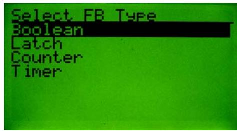
Use the **INC/DEC** keys to select the new function block type. Press the **Enter** key when the desired function block type is selected. The following screen will appear (the Boolean type screen is shown below. Other similar screens appear for other function block types.)
