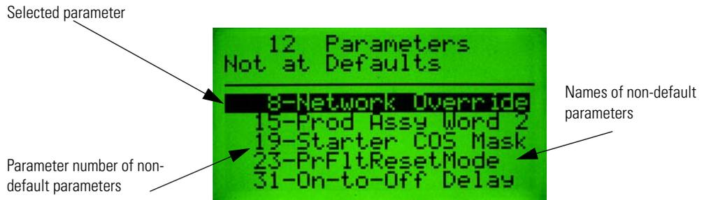
When accessing parameters found by the Search function, the format of the parameter screen will be similar to a Parameter Edit Screen with a few changes. The title line will say "Non-Default Parameter", and when **Inc** or **Dec** is pressed, only the parameter found in the search will be displayed.
