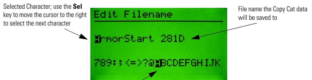
Use the **Inc/Dec** key to move the cursor to change the character. The numeric keypad can be used to enter a number into the file name
