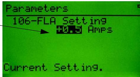
Pressing a numeric key will display an edit box to enter a new parameter value
