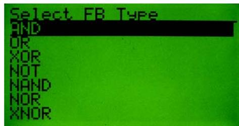
Use the **INC/DEC** keys to assign a type to the new function block. Press the **Enter** key when the desired type is selected. The screen should now display a new function block of the selected type:
