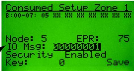
The following screen shows that byte 0 and byte 2 of the I/O data from node 5 are mapped to the ZIP data table. To accomplish this the IO Msg field must be mapped to the value of "00000101". Press the **Enter** key to edit the IO Msg field value. After editing, the value the screen will appear as follows:
