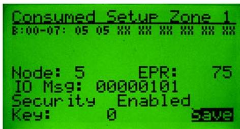
When performing a Save, all the configuration data for all Zones is saved. The Save field will disappear after the save is completed
