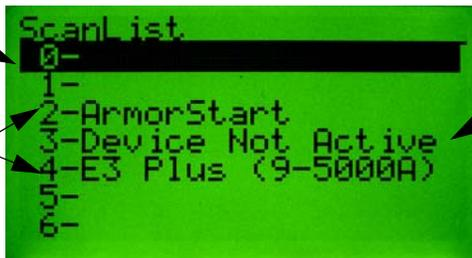
A node with errors. The error name and error number will be displayed every other second when these nodes are selected
