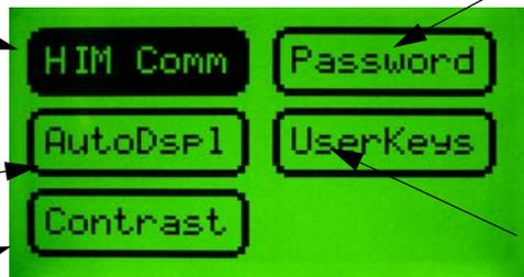
Configures the operation of the User Keys: F1, F2, F3, F4 and Reset
