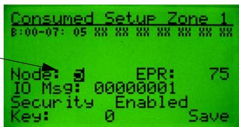
The following screen shows the EPR (Expected Packet Rate) field highlighted:
