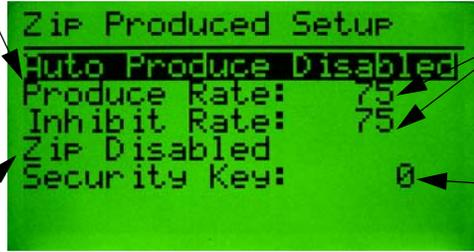
Produce Rate is the cyclic rate at which this device will produce data. Inhibit Rate is the minimum time between Change of State I/O data productions. Both values are in milliseconds.
