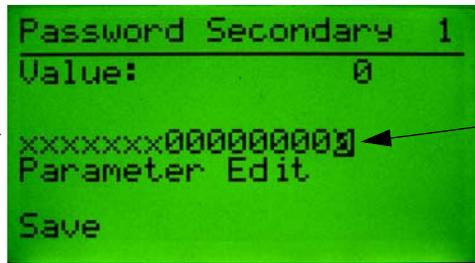
Bit Field selected. Use the **Left/Right** arrow keys to move the cursor to the next bit. This screen shows bit 0 selected.
