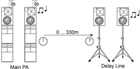
The 'external' mode supplies the delayed audio signal on the DDMs line-out. The speaker itself works without delay. This mode was created for users which want to use i.e. passive PA speakers together with an power amplifier as delay systems.
