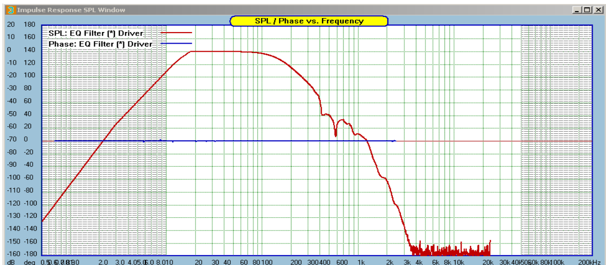
Figure 20. Complete transfer function of the subwoofer channel.
