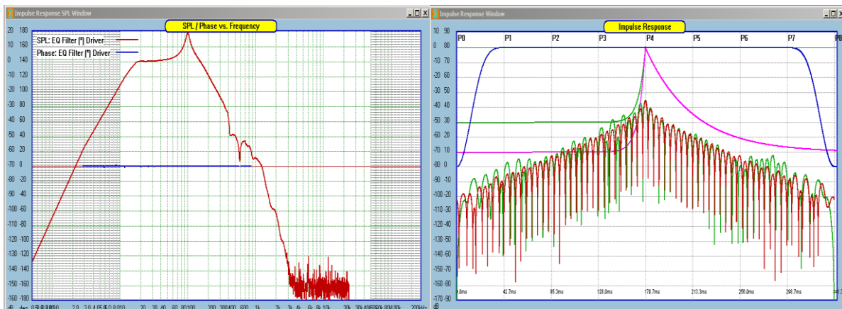
Figure 26.Pre- and post-ringing of a peaking filter convolved with a driver.
