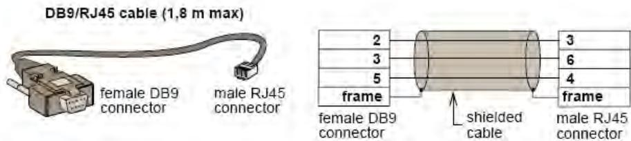
Connect the card to a computer equipped with a hyperterminal type emulator. The serial link must be set at 9600 baud, 8 bits, no parity, 1 stop bit, and without flow control.
