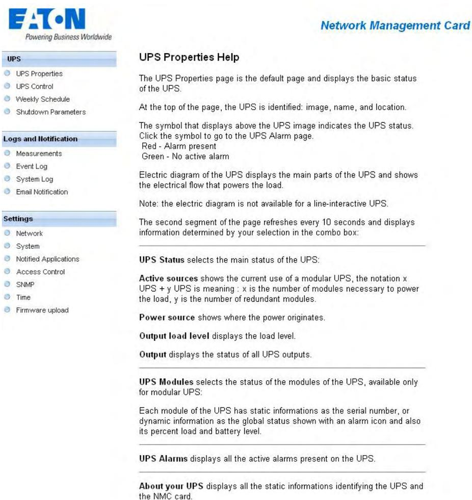
The screenshot shows the Eaton Network Management Card interface. On the left is a navigation menu with three main sections: **UPS**, **Logs and Notification**, and **Settings**. The **UPS** section is expanded, showing sub-items: UPS Properties (selected), UPS Control, Weekly Schedule, and Shutdown Parameters. The main content area is titled **UPS Properties Help** and contains the following text:
