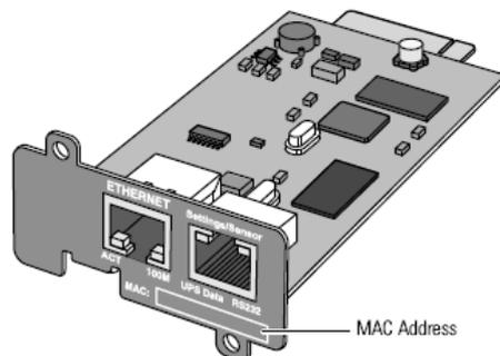
Insert and tighten the card's retaining screws
