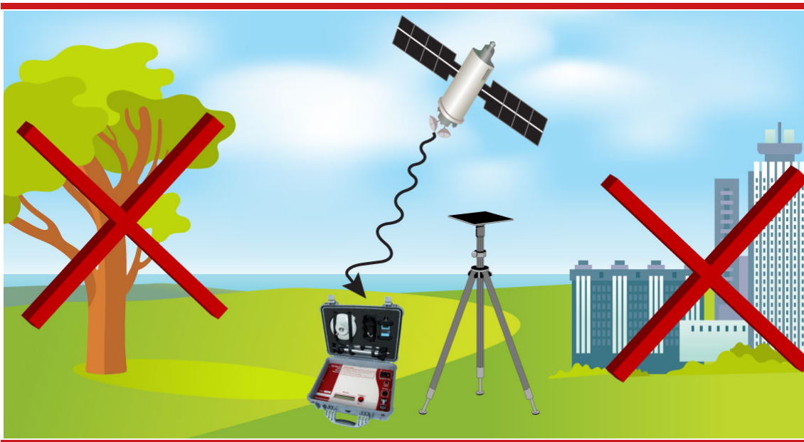
Figure 3. RT-Base Location away from Buildings, Trees and Reflective Objects
