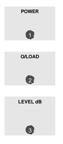
When pressing the power button, AC mains is applied to the unit. The red led below the power switch illuminates as you switch on the apparatus. The fail safe relays will open, switching the filters between the input and the output of the unit. When switching power off, the fail safe relays will link the input of each
