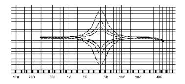
Because of this 'constant Q' circuitry, filter response does not broaden at low cut or boost settings (fig 1.2). In this way filter interaction is minimised and the 'graphic' qualities of the equaliser preserved.
