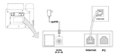
You can connect the phone to the AC Power directly by using the power adapter.
