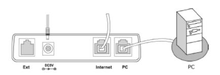
The phone can also share the network connection with other network devices, such as Computer. Connect the phone's PC Port and Computer's Network Port together using an Ethernet cable.
