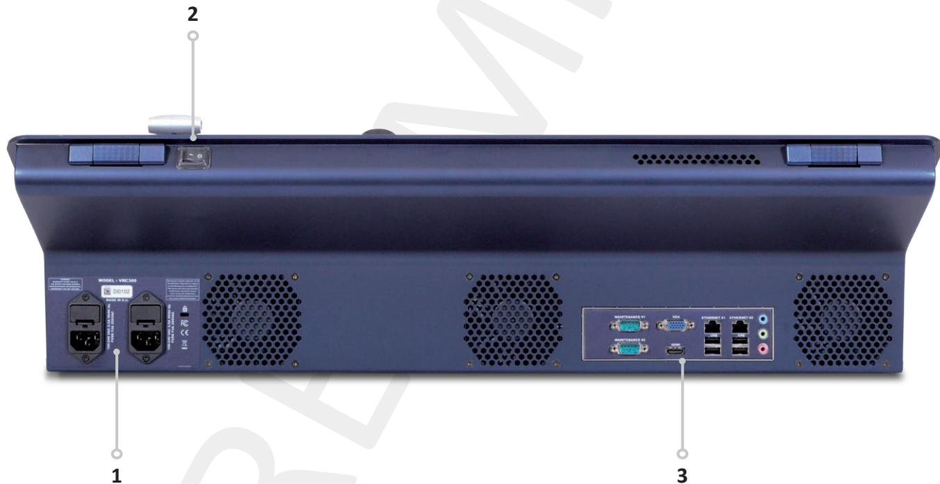
**1. Power Supply:** Dual, redundant power supply with fuse as standard equipment.
