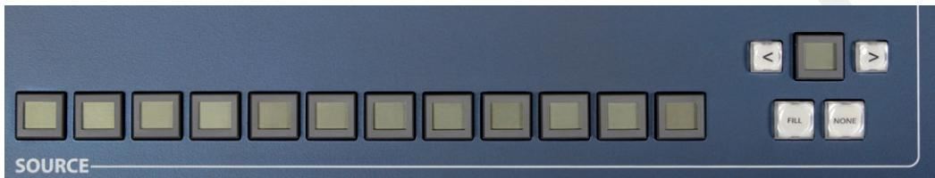
Use the left/right arrow to navigate into the source page. Then simply press the desired source in order to fill the layer.
