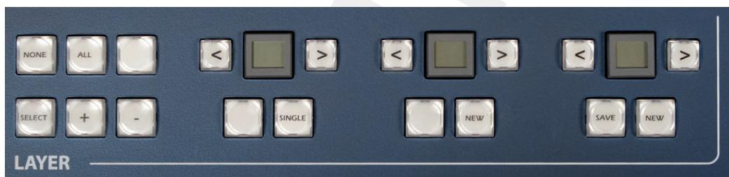
navigate to the desired screen, pressing the large LCD button at the center of this group will select all of the layers on the desired screen on Program or Preview.
