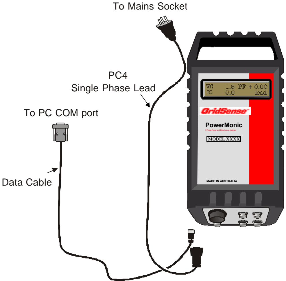
Fig 16 – Connecting the PowerMonic to the PC
