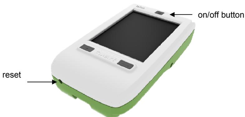
**Turn on** the Tellus smart by pressing the *on/off button* until the screen turns on.
