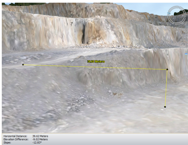
Figure 99 - The horizontal distance between two positions
