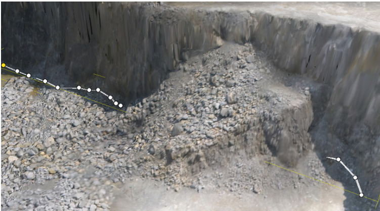
Figure 48 - Example of a bottom bank breakline where a pile of debris has been excluded. Vertices have been placed before and after the pile, not on top of it.
