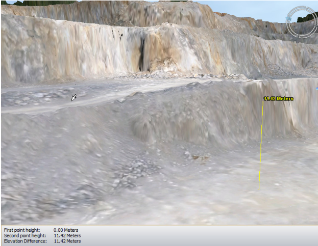
Figure 101 - The vertical distance between two positions
