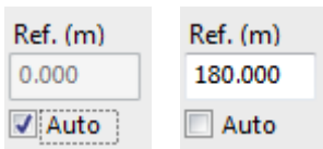
Figure 60 - Elevation reference level set to automatic (left) or manual (right)
