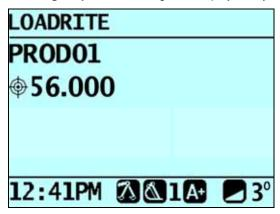
As you lift a weight, the target weight is displayed along with the current lifted weight and the potential weight if the lift is added.
